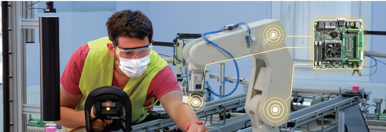
Industrial robots with collaborative applications are becoming a critical asset to the manufacturing sector. The requirements of collaborative applications for industrial robot is to reach safety performance level up to SIL2 according to IEC 61508, or Cat.3 PL=d according to ISO 13849-1.
