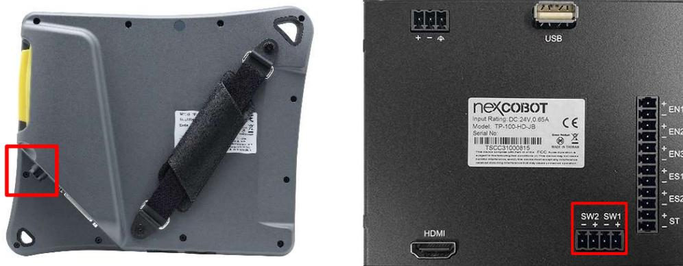
The switch button connects to SW1 at the back of the junction box. When the switch button is pressed, the SW1 status will change from Normal Close (NC) to Normal Open (NO).
