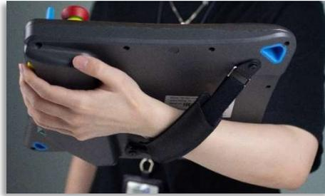
The TP-100-2 teach pendant is designed to operate in a horizontal / landscape format. When operating the device, make sure to connect all necessary cables from the teach pendant to the host computer.
