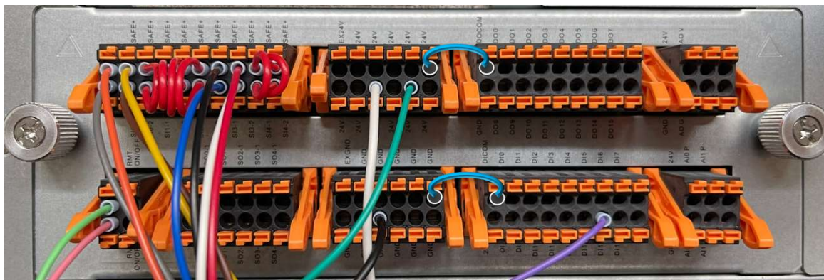
Connecting junction wires (PNP type) to TM control box
